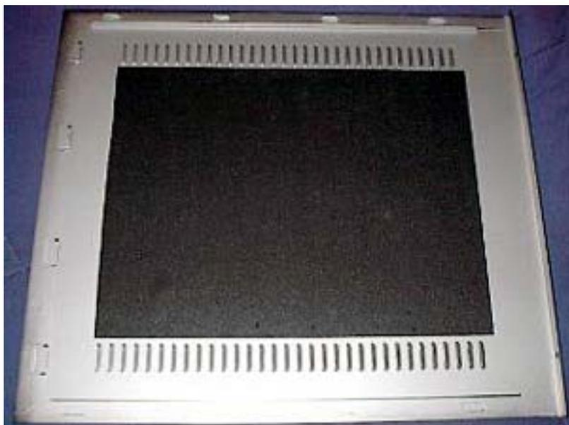
After installation of the VBlock VB-2 SSDM, which consisted of ~ 50% coverage, the meter read 66db. While 2db is not an earth shattering reduction it was noticeable. Keep in mind if I didn't have a window in one of my side panels and could have achieved 80% or 85% coverage I would imagine the difference would have been on the order of a 4 or 5db sound reduction. I also noticed no case temperature increases with the VBlock VB-2, that was certainly welcome news.
