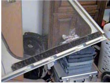
After you have cut the hole in the case, attach the plastic weather strip so that the edges look smooth and nobody will cut themselves on the edge. Then cut the plexi to the approximate size of the hole (a little larger to accommodate for the velcro strips) and stick the glass to the inside of the door. These pics illustrate how the glass attaches, and how I had to cut the glass around the lock mechanism. (a little sloppy, but who cares - it looks GREAT from the outside!!!)
