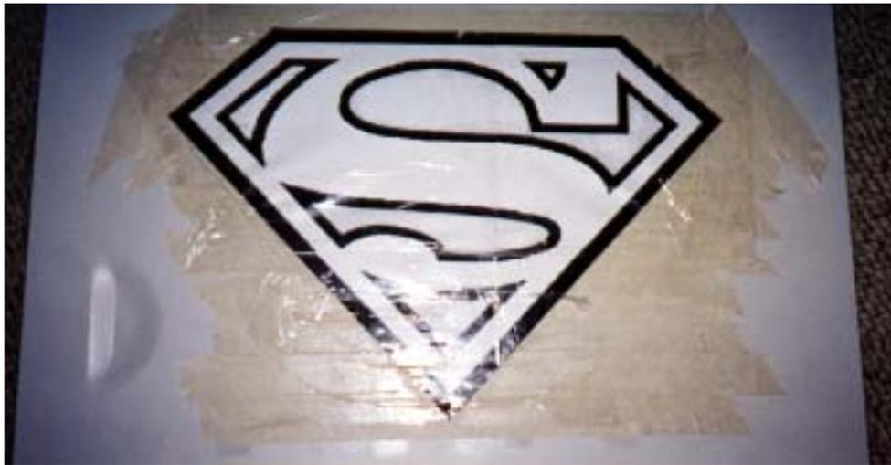
I cut along the edges of my pattern till I could see the metal all along my cut and then I removed the printed pattern and the clear tape leaving behind the masking tape. You can still see the pattern since I've already cut through the masking tape and into the metal. After a while the printed pattern was just getting in the way since it wasn't glued down just taped around the edges so it bunched up a bit.
