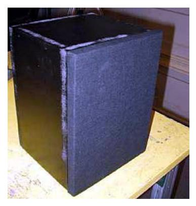
Once again, the gray stripes caused by the cut edges soaking up the paint is probably more pronounced in the pictures than in real life. They are noticeable but it doesn't really detract from the look of the boxes in place. Here's a picture of one of the satellites in place; they wired directly into the subwoofer amp powered output terminals.
