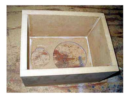
I used the same assembly technique on these boxes as I did on the subwoofer - I assembled the boxes first using some 4d finish nails and then installed a couple of 1-5/8" drywall screws on each edge for strength. Make sure that you pre-drill any screw holes (edge, at the speakers, etc.) to avoid splitting the material.
