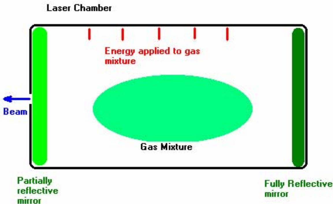
Basically, we fill a chamber full of the gas mixture, apply an electric field and the photons emitted from the excited atoms start to resonate between two mirrors, one partially reflective. The resonating light partially escapes the chamber through the partially reflective mirror; this 'escaped' light is our laser beam! The light remaining in the chamber stimulates the emission of more photons from the gas atoms.
