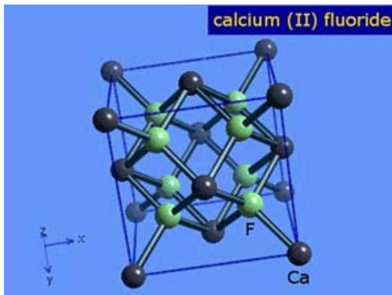
An additional major concern is the resulting compaction of the optics. Compaction changes the refractive index (air or H<sub>2</sub>O has the index of 1) of an optical element and also the thickness. This change causes lightwave aberrations and deteriorates the microlithographic process results. The solution: Replace fused silica optics with Calcium Fluoride (CaF<sub>2</sub>) optics where it is critical within the optical path (projection optical lens).
