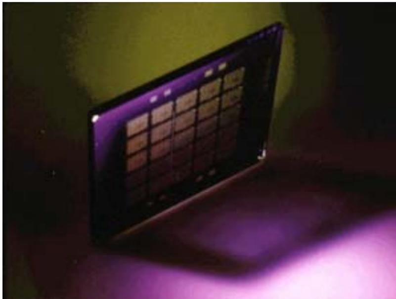
Reticles are an integral component in the lithographic process of semiconductor manufacturing. High-purity quartz or glass plates containing precise images of integrated circuit layer. Each layer of a microchip will require a different reticle containing the desired image. These images are optically transferred onto the silicon wafers as discussed previously in chapter 2.
