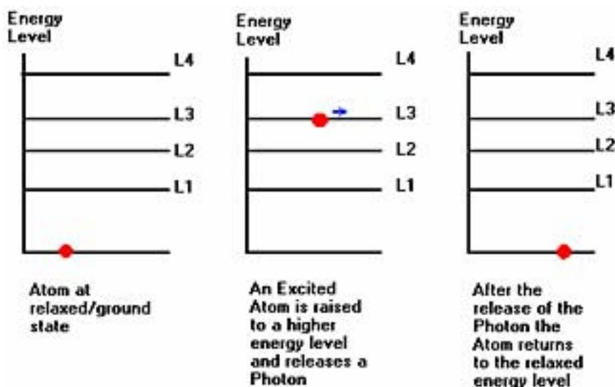
The emission we are referring to is a characteristic of atoms to emit photons ("particles" of light) under certain and reproducible situations. Chemical or electrical influences can be these said situations. To cause a
