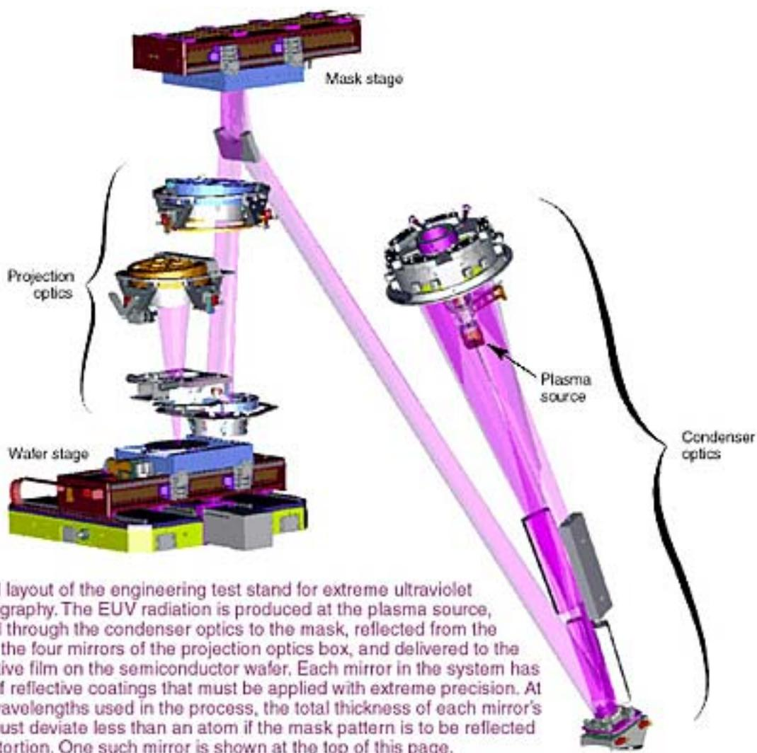
A proposed EUVL microlithographic system would use a laser-produced plasma to supply the EUV radiation source (80W-100W of power needed). The solutions to provide such an energy source are either huge magnetic field created currents or coupling the power of multiple lasers. These power sources will generate large amounts of heat with temperatures exceeding 1000°C.
