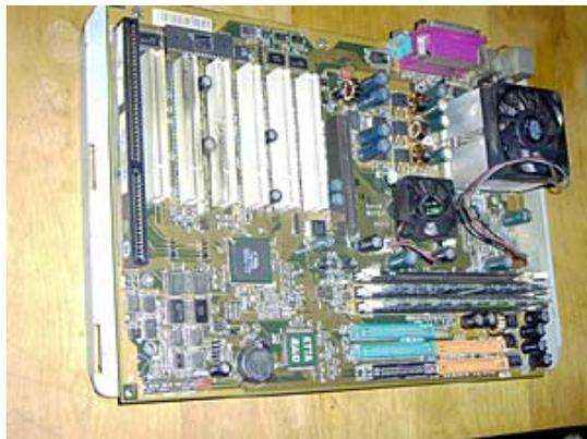
Once everything had been pulled out and cleaned, I took the old motherboard off the tray and put the new one on. This being an older case, the mobo tray, a perfect fit for the old motherboard, was on the small side for the A7N8X.
