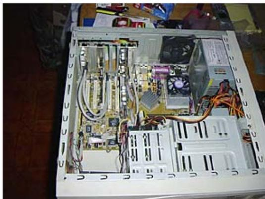
There! I don't have any shrink-wrap or wire wrapping, so the PSU wires were routed as best as possible and the unused wires tucked up at the top. I used the IDE and floppy cables that came with the motherboard so I could do "ribbon cable origami" instead of my old "cut up and electrical taped" cables. I was quite proud of myself in this, and it added an hour or so to the total install time. But I was done!
