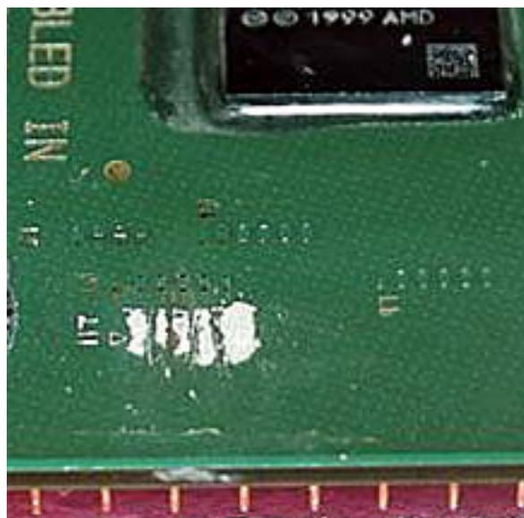
There are some rules to follow when connecting the dots... you must not cross-short, you must fill in the pits between the dots and you must not allow the conductive ink to touch any of the ground points on the CPU. Why? 'Cause I said so! Now stop asking silly questions! Now that that's settled; What's a ground point? Every
