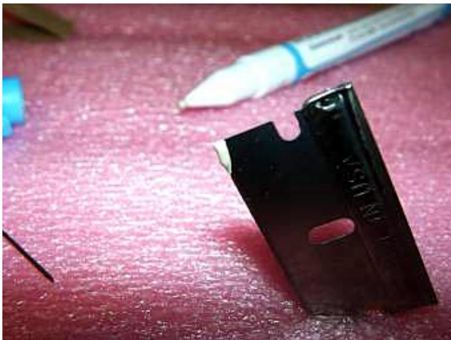
As you can see I favor a razor since it is easier to control for my trembly hands. I dip the edge in the silver ink and lightly drag it between the dots... it works for me. I then use a pin to separate cross-shorts... I simply wait for the ink to get tacky and then separate the bad spot with the pin... leaving a clear channel between shorted bridges.
