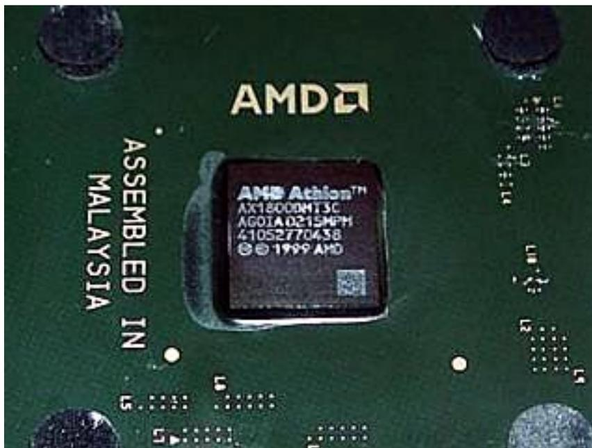
This is an XP1800+ that has had the pits pre-filled with my favorite goop... Liquid paper; pits are the laser cuts AMD has made between the dots in order to discourage people from messing with the hardlocks. If you do not fill the pits in you will short the dots to the grid below the substrate and mess up the process so: Fill In The Pits! Now lets goto OCinside and [look at the schematic our desired alterations bring up.](#)
